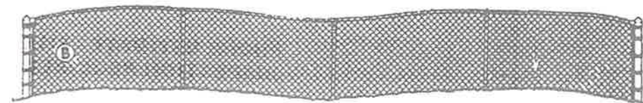
B Fence following grade, rolling terrain
